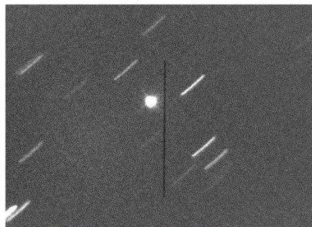
10 sec. exposure with the spectrograph guiding camera Thank to a special programming of alt-az telescope, the asteroid is a fix object The vertical line is the 23 microns spectrograph entrance slit
