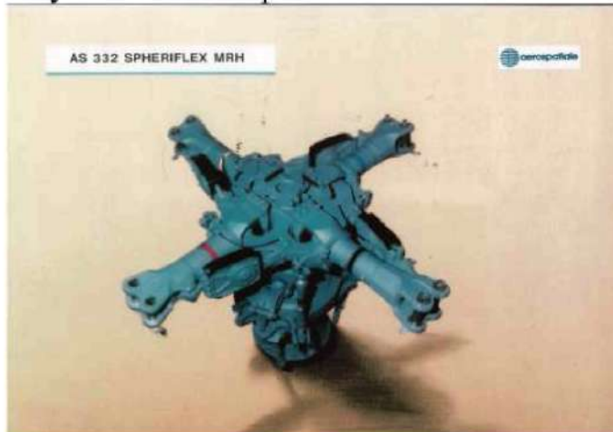
Moyeu Sphérflex AS 332
